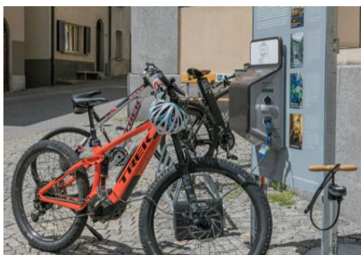
Figure 7: example of e-bike charging stations (from [9])
